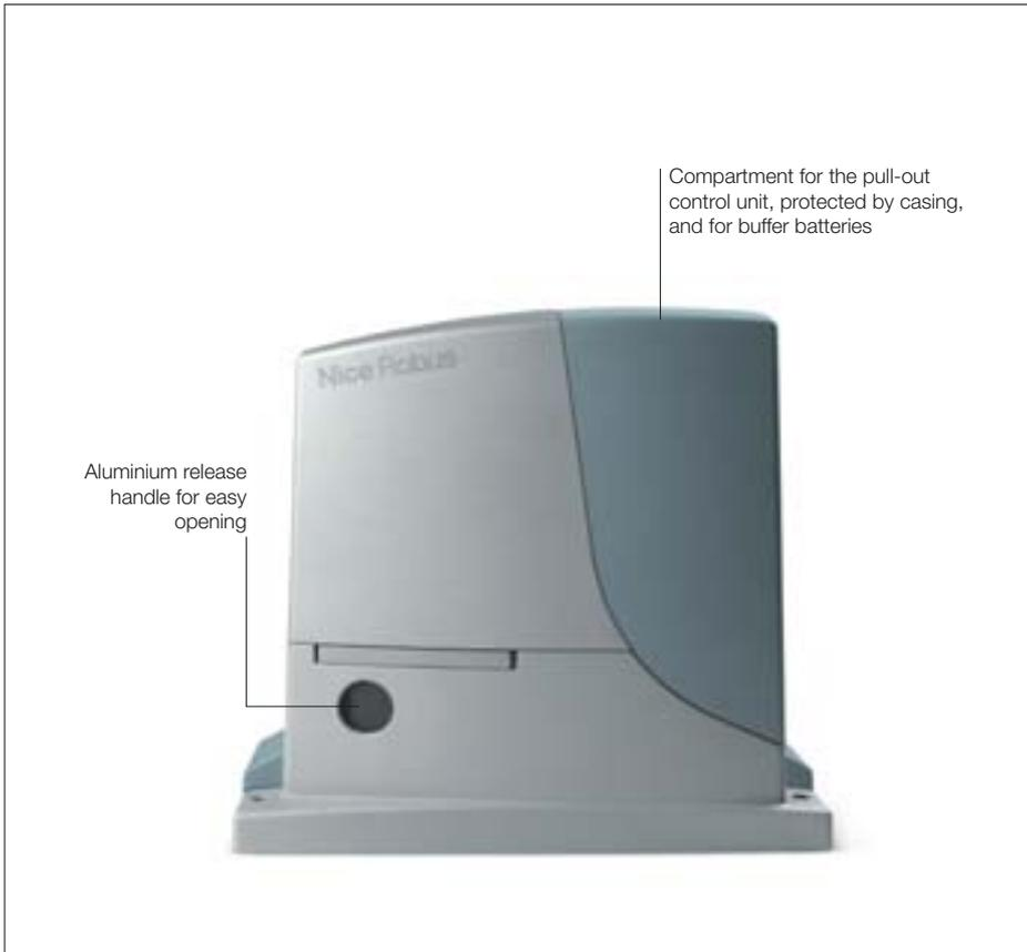
**For sliding gates weighing up to 600 kg (RB600) and up to 1000 kg (RB1000). Electromechanical gear motor with Nice BlueBUS technology. Versions with electromechanical limit switch (RB600/RB1000) and with inductive limit switch (RB600P/RB1000P).**
