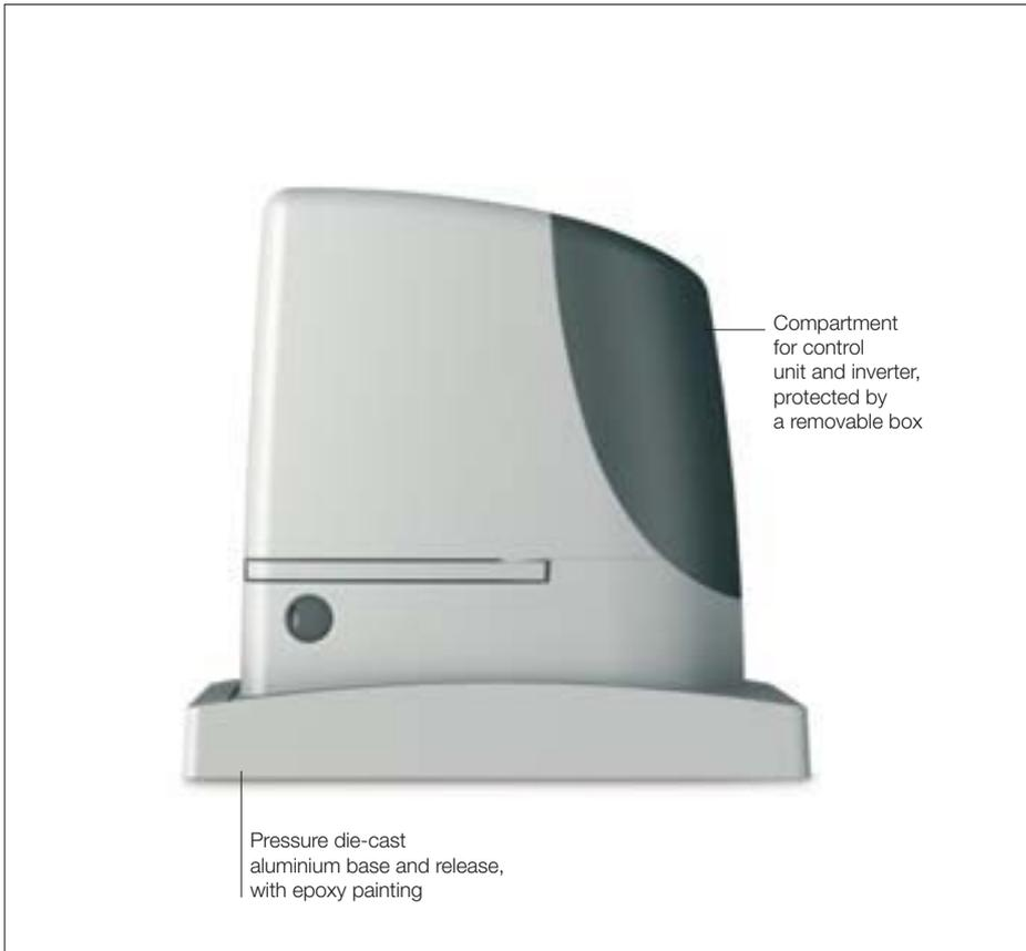
**For sliding gates weighing up to 1800 kg (RUN1800) and up to 2500 kg (RUN2500), with Nice BlueBUS technology. Ventilated motor with inductive limit switch (RUN1800P/RUN2500P) or electromechanical limit switch (RUN1800/RUN2500/RUN2500I).** Suitable to operate in extreme conditions, in systems for intensive use.
